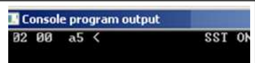
KIM Uno over the serial port: using Mode 1 (emulation of onboard 6 digit LED display)
